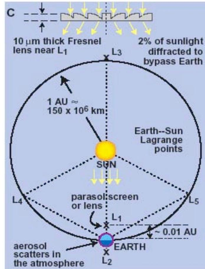
**(Left) Wireless power from space** could enable developing nations to avoid fossil-fuel-based industrialization. Ultralight large SPS aperture antennas and other components could be fostered by nanotechnology. **(Right) Deflecting sunlight** with a 2000 km flat lens at the  $L_1$  Lagrange point or intentional aerosol injections to the stratosphere are potential “worst case” mitigators of global warming.
