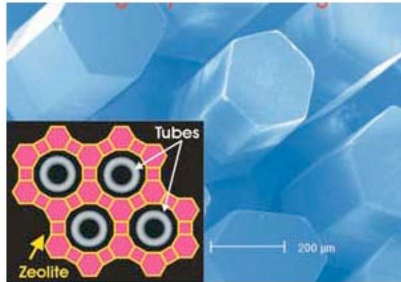
**TINY TUBES** Superconducting nanotubes inside zeolite pores (inset), against backdrop of zeolite crystals.
