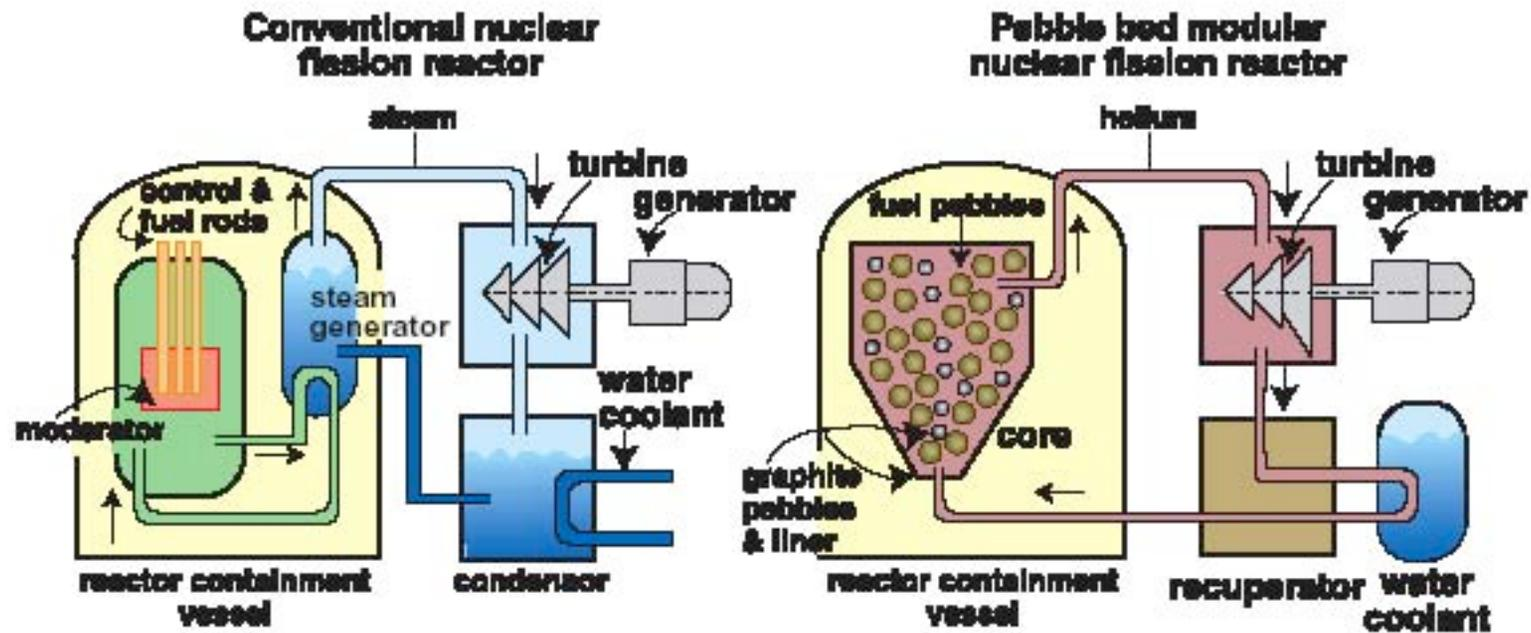
(LEFT) The conventional light water reactor (LWR) employs water as both coolant and working fluid. (RIGHT) The helium-cooled, graphite-moderated, pebble bed, modular nuclear fission reactor is theoretically immune to loss of coolant (TMI) and criticality (Chernobyl) accidents.
