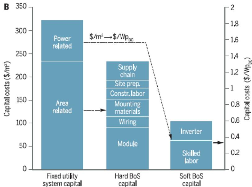
The above figure of a utility-scale PV system from the Lewis (2016) paper shows how some components of the system scale with the required array area – such as installation labor (middle column), while some do not – such as those tied to the power produced (in right column).
