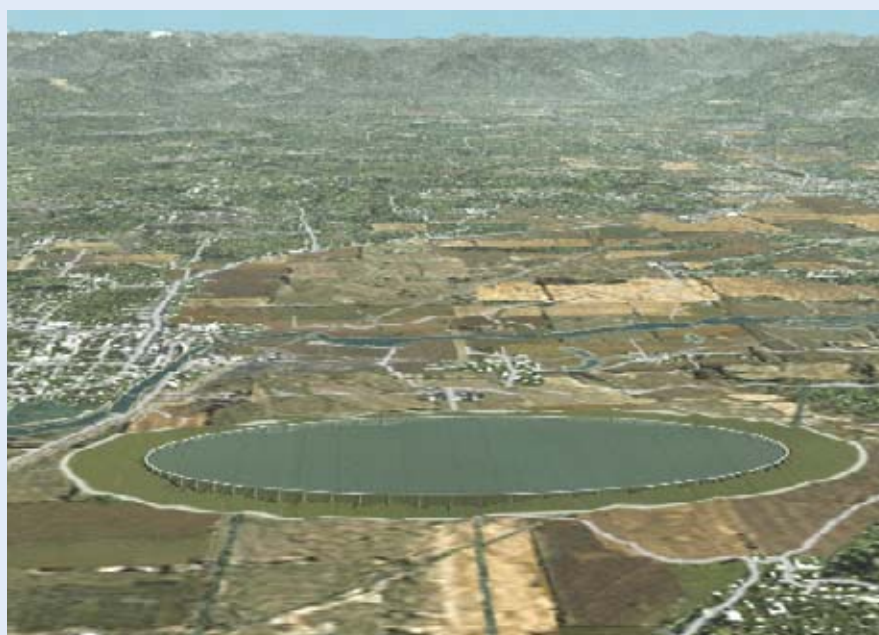
Private companies such as PowerSat Corp. have proposed erecting large rectifying antennas in order to collect microwave energy that is beamed from orbiting power stations.
